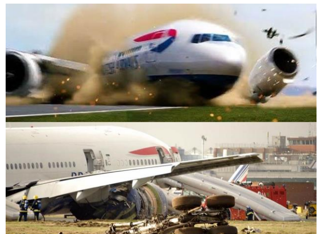
Figure 3. A Boeing 777 crash-landed on a runway in 17 January 2008 demonstrating the impact and damage mostly on the “below the wing” turbofans.
