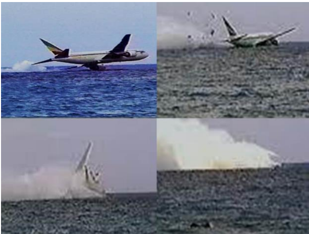
Figure 2. A Boeing 767 crash-landed on the sea in 23 November 1996 demonstrating how “below the wing” turbofans may cause an aircraft to be less seaworthiness.
